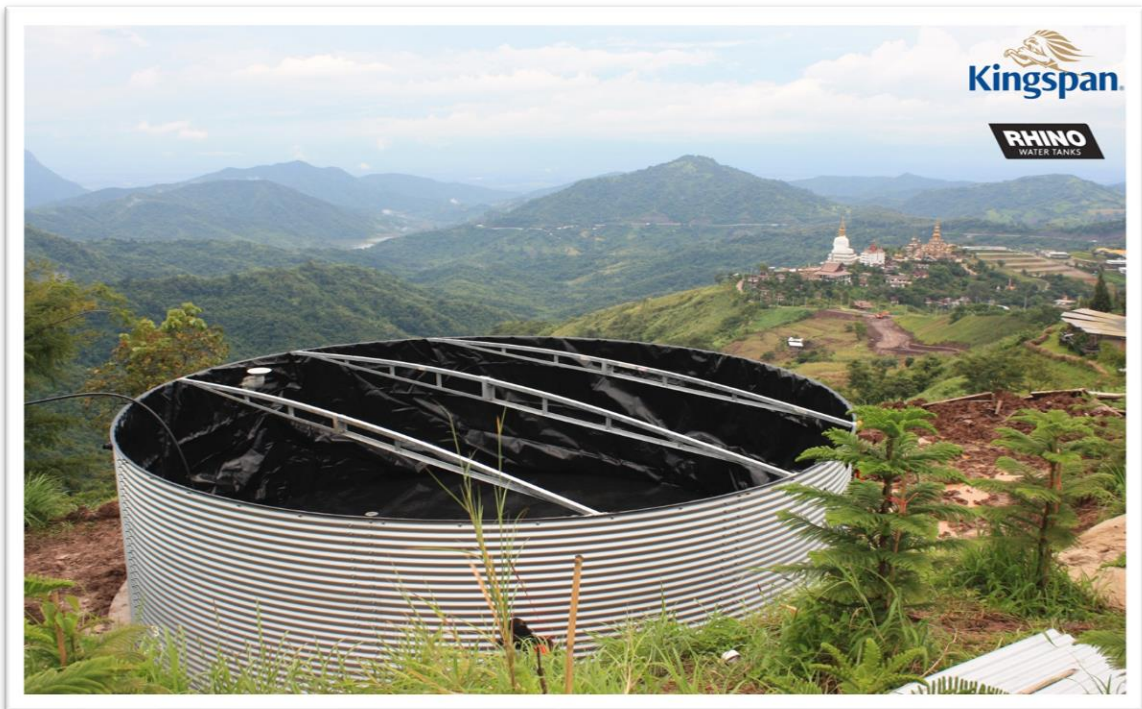
Pino Latte RCT100-22 (104,305 L) Khao Kho, Phetchabun Diameter: 7.768 m H: 2.20 m Clean water storage for the client's coffee shop business. The daily usage can be up to 40,000 liters of water per day and the supply can be intermittent. The tank provides approximately 3 days of water storage.
